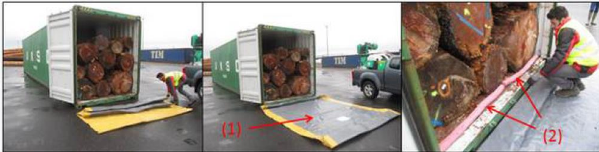
installation of the hermetic recovery tarpaulin (1) and absorbent draught excluders (2)
